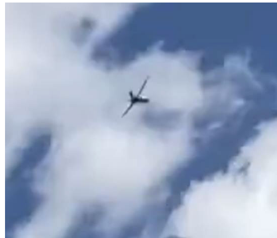
(b) Photograph of the MIT Firefly air vehicle in-flight, cruising at roughly 40 m/s.
